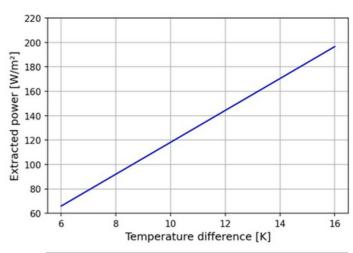
$\Delta T = T_{in} - T_{wall}$  = Temperature difference  $T_{in}$  = Fluid inlet temperature  $T_{wall}$  = Wall temperature
