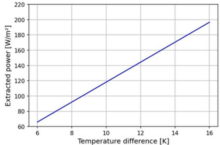
$\Delta T = T_{in} - T_{wall}$  = Temperature difference
